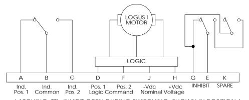
LATCHING, TTL, INHIBIT OPEN DURING SWITCHING, SHOWN IN POSITION 1
