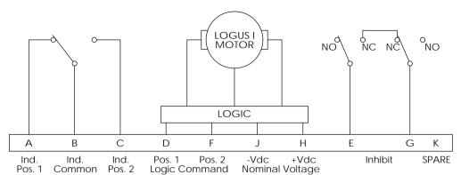
LATCHING, TTL, INHIBIT CLOSED DURING SWITCHING, SHOWN IN POSITION 1
