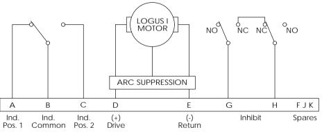
FAILSAFE, INHIBIT CLOSED DURING SWITCHING, SHOWN IN POSITION 1, DE-ENERGIZED
