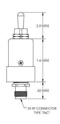
Frequency (GHz) DC to 4 4 to 8 8 to 12.4 VSWR (Max.) 1.2:1 1.4:1 1.5:1 Insertion Loss (Max.) 0.35 dB 0.5 dB 0.2 dB Isolation (Min.) 70 dB 80 dB 60 dB Power (Max.) 100 WCW 80 WCW 75 WCW
